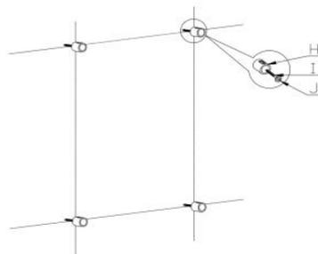
3. Screw the 4 bracket inserts (support) into the bracket bases to the radiator using M5 screws provided (securing each with a washer).
